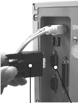
9 pin D female connector fitted to Denford machine link cable.
