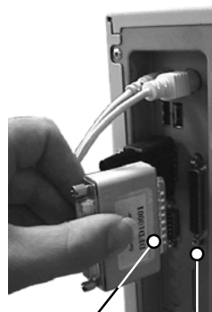
25 pin D male connector on security key (dongle).
