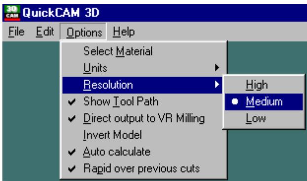
NB, changing the resolution setting will automatically re-calculate the toolpath for you if you are in this stage of the process.
