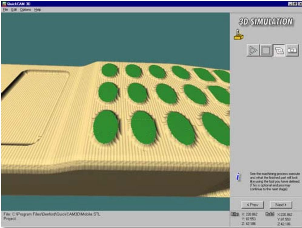
You can zoom into the model to view specific parts in detail. In the example shown above, although the buttons are fairly well defined we could trace back to previous stages, change the tool stepover to a smaller (finer) percentage and run the simulation again to help remove the rounded edges. The green colours show areas of the billet that have not been machined.
