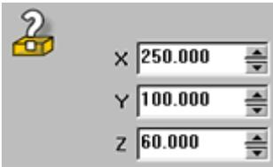
You enter the dimensions of your billet using the X, Y, Z readout panel, in the top right corner of the screen. Click in each readout box and enter the required dimension value. The billet dimensions are stated in millimetres or inches, depending on your "Options|Units" setting. Alternatively, clicking [Up] and [Down] nudge buttons, positioned on the far right of each X, Y, Z readout box, steps the selected dimension up or down by one unit.
