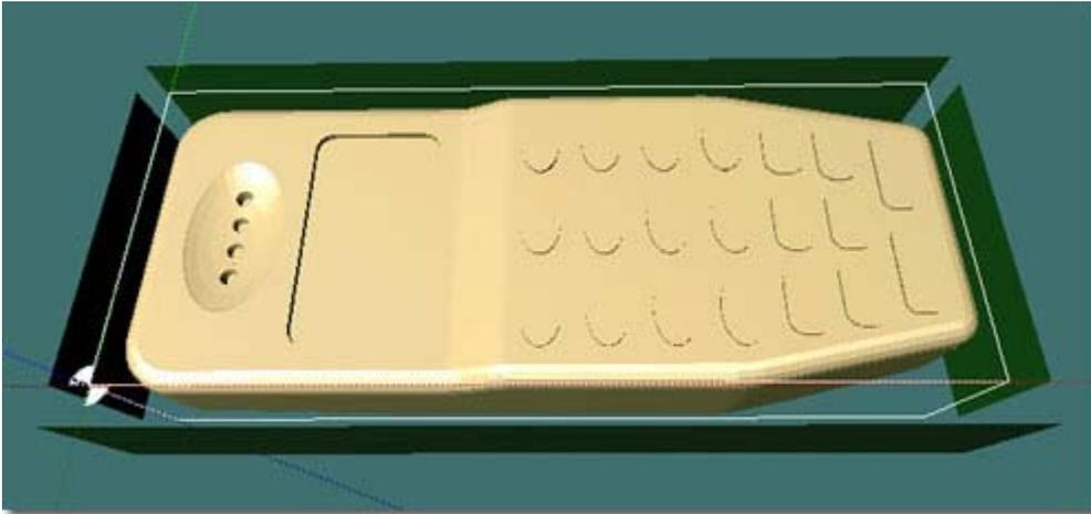
Clicking the  button will automatically create a billet size identical to the boundary size of your 3D model. You can still use the [Up] and [Down] nudge buttons to change these billet dimensions.
