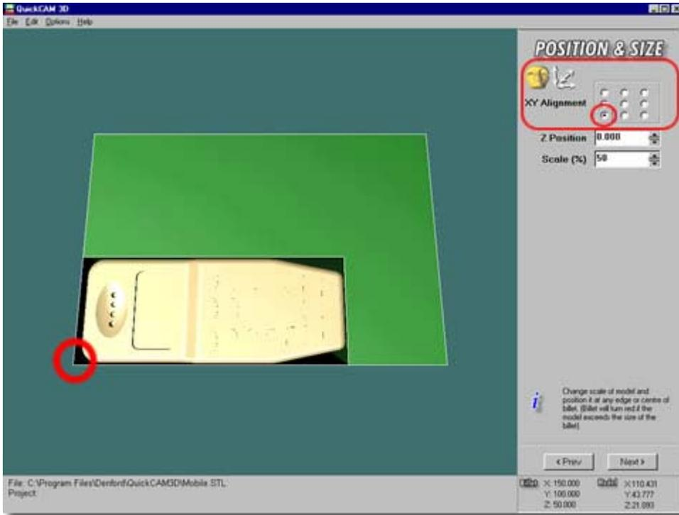
To reposition the model in the billet, click inside the appropriate circular white marker. The black dot will transfer to the chosen marker and the model will shift position within the billet. In the example above, the model has been shifted to align with the front X and left Y edges - the front, left corner of the billet.
