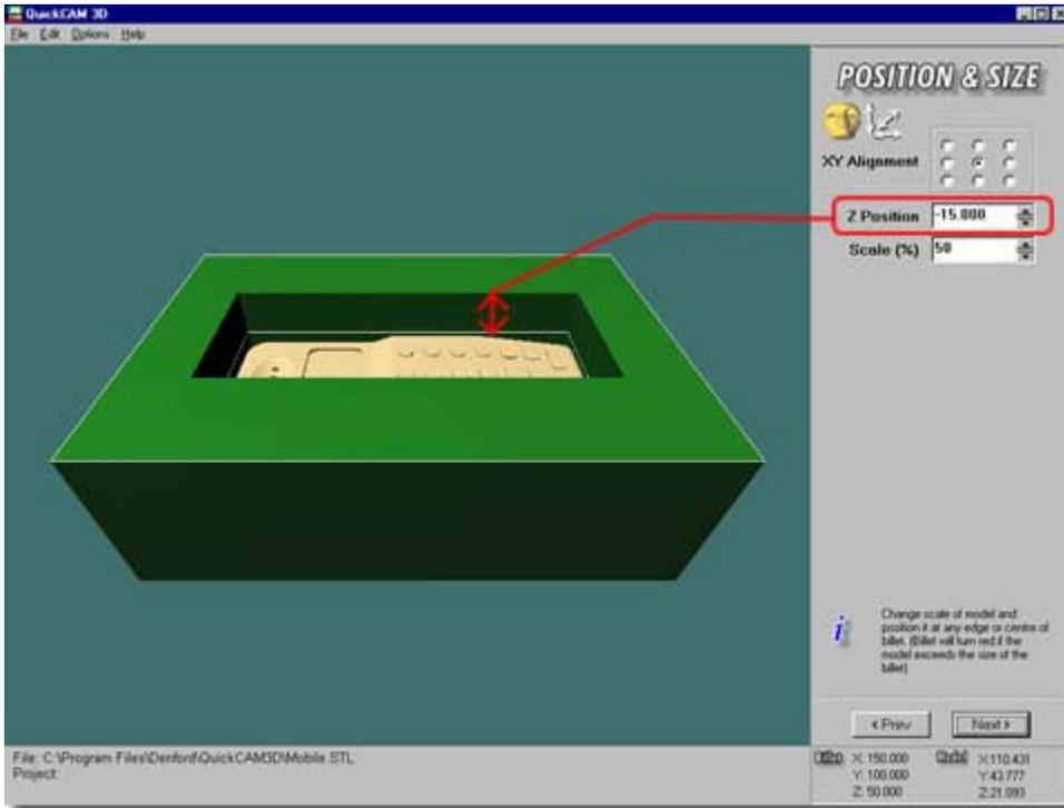
The model is raised or lowered in the billet by over typing with the required value, or by using the [up or down arrow] nudge buttons. As the value changes, the model position will update in the main graphic panel. Positive values raise the model whilst negative values lower the model.
