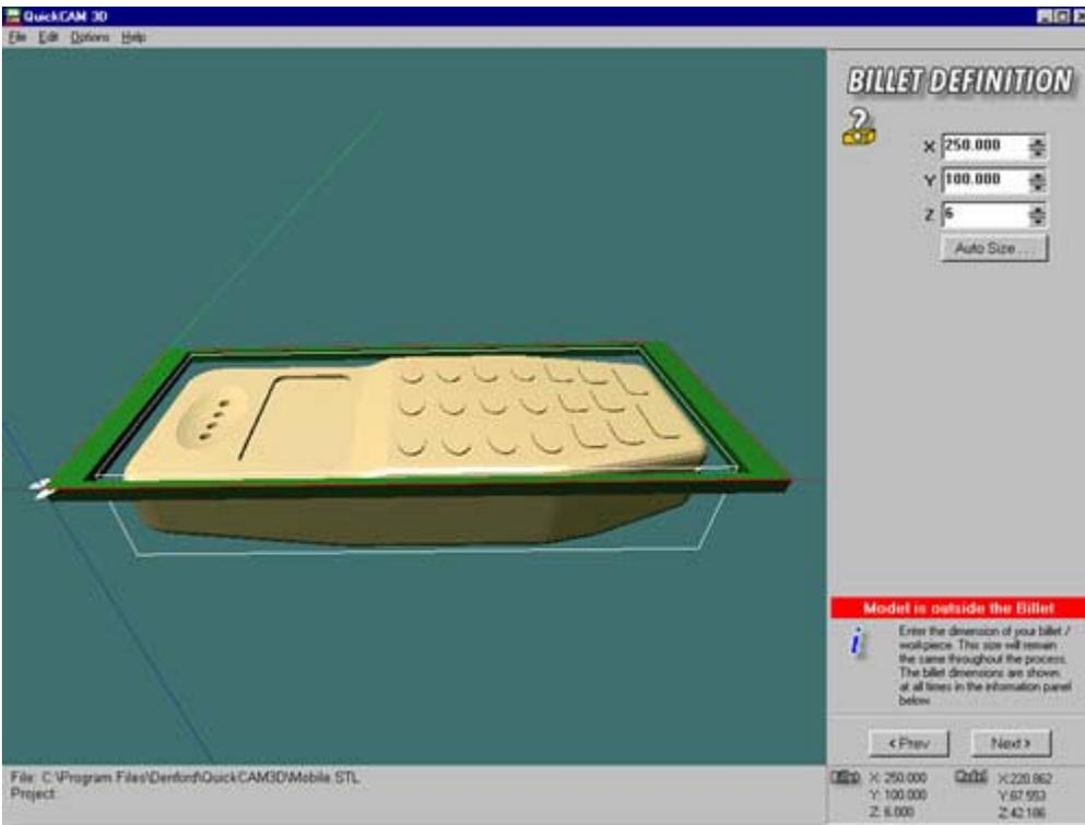
As each dimension is entered, the green block representing the billet will be updated on the view of the 3D model. Notice that a warning message appears whenever you enter a dimension that is smaller than 3D model size.
