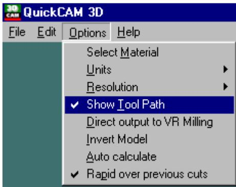
For most types of model, it is best to select medium resolution (default) for the calculation. This option gives a good finish to the calculated toolpath, without taking too long to process. However, you may find you want a better quality finish on the finished part. For this you would select **High** resolution. Select **Low** for very large models, or ones that take a long time to calculate:
