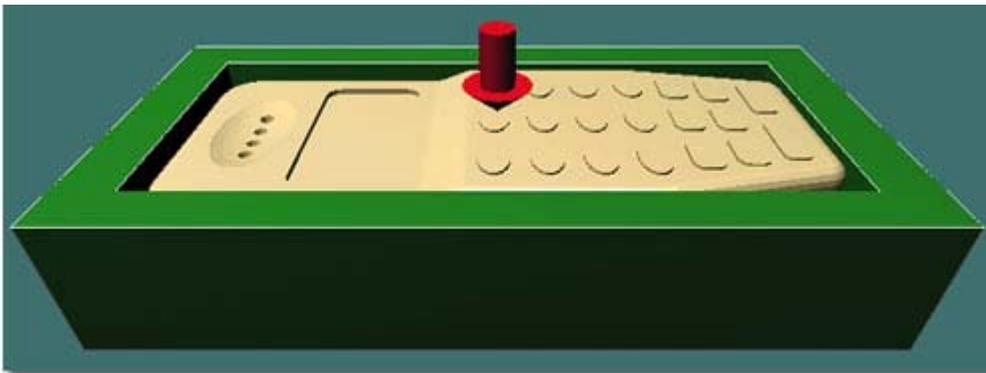
Using the [Up] and [Down] nudge buttons, positioned on the far right of each X, Y, Z readout panel, rotate the 3D model in 90° steps to best fit inside your CNC machine - imagine the view you are seeing is the view through the front window of your CNC machine. Usually, you want to align the longest side of the 3D model with the longest axis of your CNC machine (most commonly the X axis).
