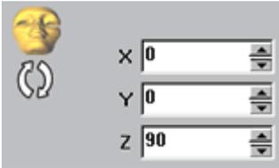
The red arrow can be moved around the faces using the [Up] and [Down] nudge buttons, positioned on the far right of each X, Y, Z readout panel. Each click of a nudge button will step the red arrow 90 degrees across the selected axis.
