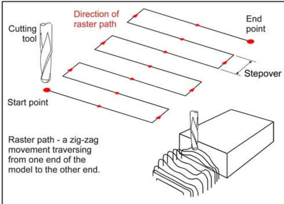
The value entered in the 'Stepover' panel defines how much the tool moves before starting the next line on the raster path, or zig-zag. This value is calculated as a percentage of the diameter of the tool, as shown in the diagram below.
