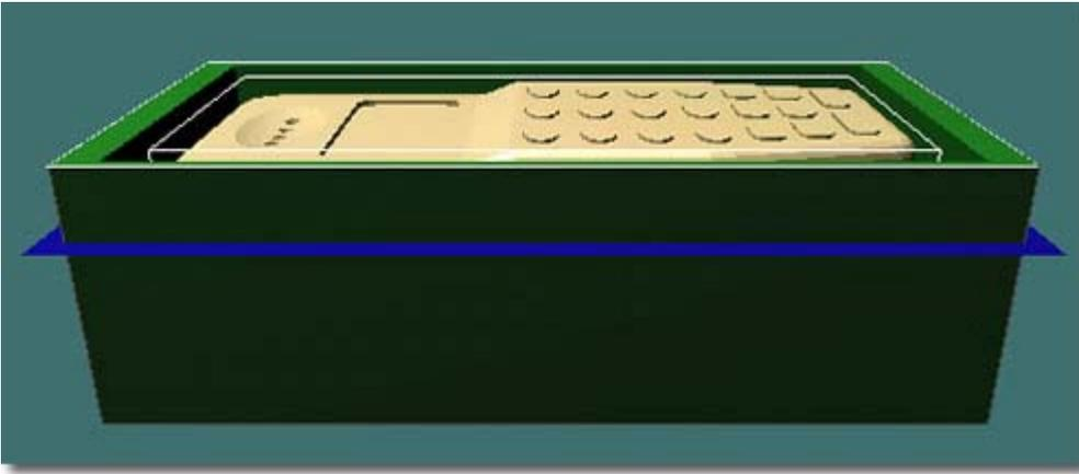
Clicking  will position the cutting plane exactly in line with the bottom surface of your 3D model, as shown below. Notice that this operation applies to the bottom of the model, not the billet.
