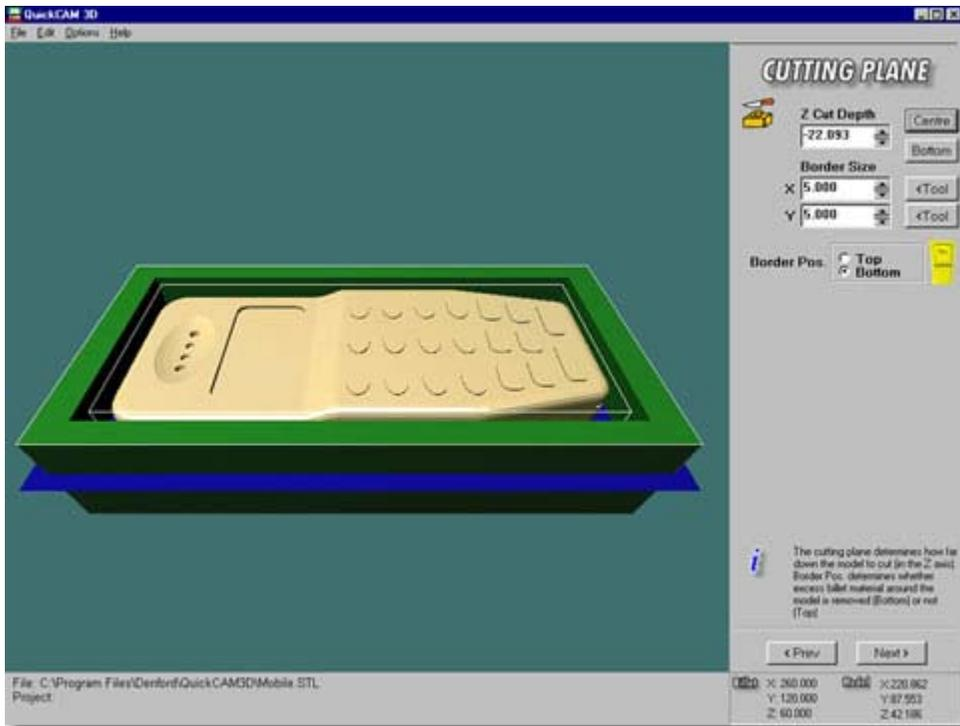
The cutting plane, shown by the blue rectangular slice through the billet and model, defines the maximum distance you want to cut into the billet. Any part of the 3D model below this cutting plane will be ignored when your CNC file is written. In other words, all the parts of your model below this cutting plane will not be machined.
