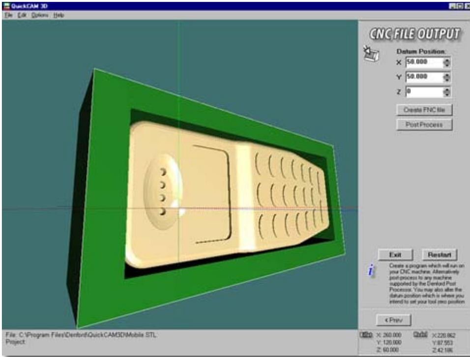
For example, you may want to move the datum to align with a specific part of the billet or a known position on a jig or fixture that you will be using on the CNC machine. Remember, the datum position you set here will need to be found on the CNC machine, when you configure your CNC machine offsets. In the example above, we have moved the datum so the zero position of the program will lie along the centreline of the Y axis, 50mm inside the left edge of the billet.
