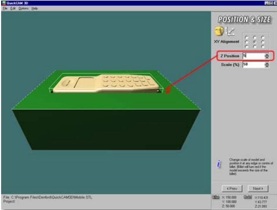
Parts of the model not contained within the boundary of your billet are highlighted. In the example above, the control panel and buttons on the mobile phone model are positioned too high - they are breaking through the upper boundary of the billet.
