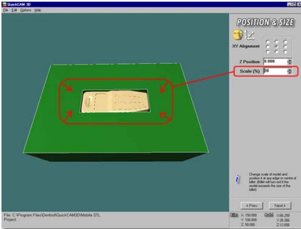
Use the Scale (%) panel to proportionally increase or decrease the size of your model within the billet. In the example above, the model has been scaled to 30% the original size.
