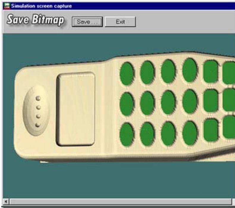
Snapshots are useful for showing how your final model may appear in a variety of different materials, or showing how your machining strategies have developed. For example, if you are unhappy with the surface finish, you could take a snapshot, then change some of the parameters in previous screens and resimulate the model, building up a portfolio to explain how you overcame these problems.
