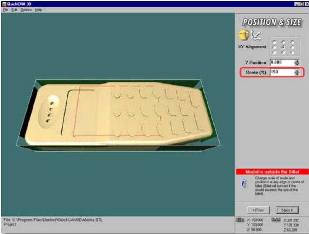
When increasing your model scale note that a warning panel will be displayed when your model size exceeds the size of your billet. In the example above, the ends of the model protrude from the billet.
