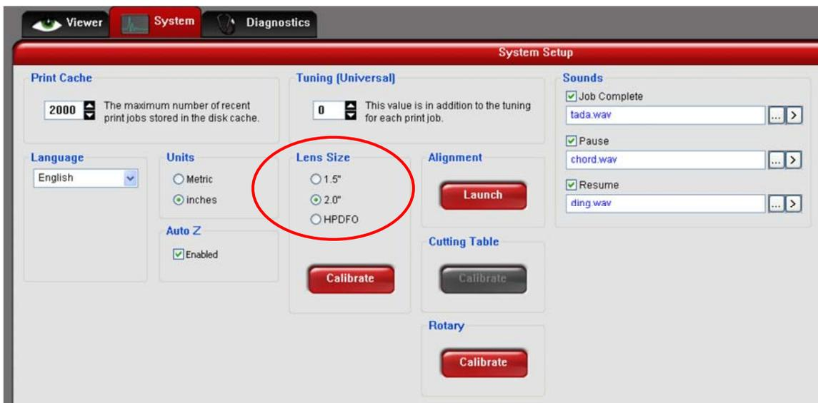
5. If you have purchased the 1.5 or HPDFO optional lens kits, calibrate the lens kit according to steps 1 through 4. Be sure you select the proper lens size from the list before calibrating.
