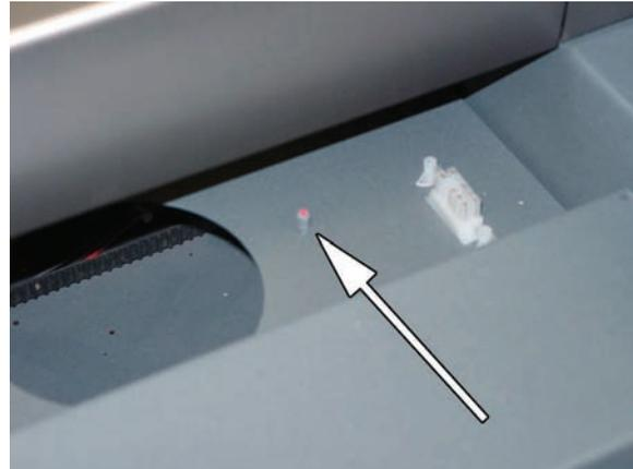
7. Proceed to the UCP and activate the focus feature on the right hand side of the Viewer Tab. Click within the focus feature and have the focus carriage move over the alignment pin as shown. Use the red LED to position the focus carriage over the pin properly. You can also use your computers keyboard to control the movement of the focus carriage when you are using the focus feature. **DO NOT** exit the focus feature yet.
