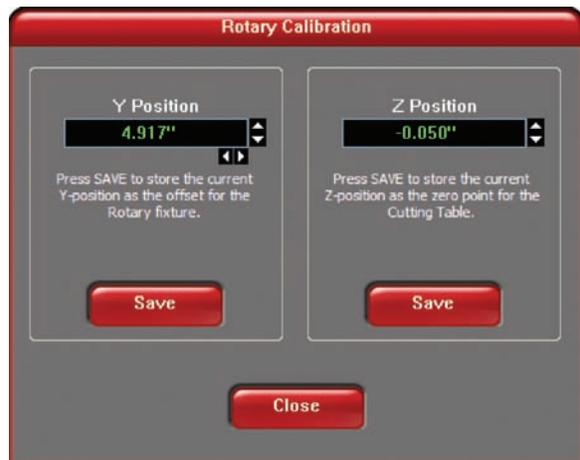
14. Once you have manually focused proceed to the System Tab and click on the Rotary CALIBRATE button. The Rotary Calibration window appears. Click the SAVE button for the Z Position **ONLY**. If it asks you to override the current position accept the new number.
