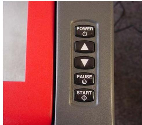
2. Using the UP and DOWN arrow buttons, either on the machine or in the UCP, bring the Z-axis table up. Using the appropriate Focus Tool for the lens installed (the standard is 2.0, other Focus Lens Kits are optional), focus directly on the surface of the table.
