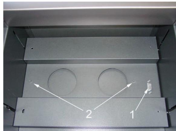
5. Inside the VersaLASER you will find the large recessed slot with a self-aligning electrical connector to the right side (1) and the two alignment pins (2)
