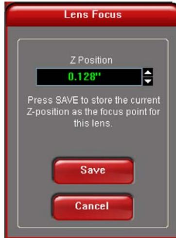
4. Click on the Calibrate button within the Lens Size box of the System Tab. The following window appears. Click on Save to accept the new Z Position. Your 2.0 Lens has now been calibrated.
