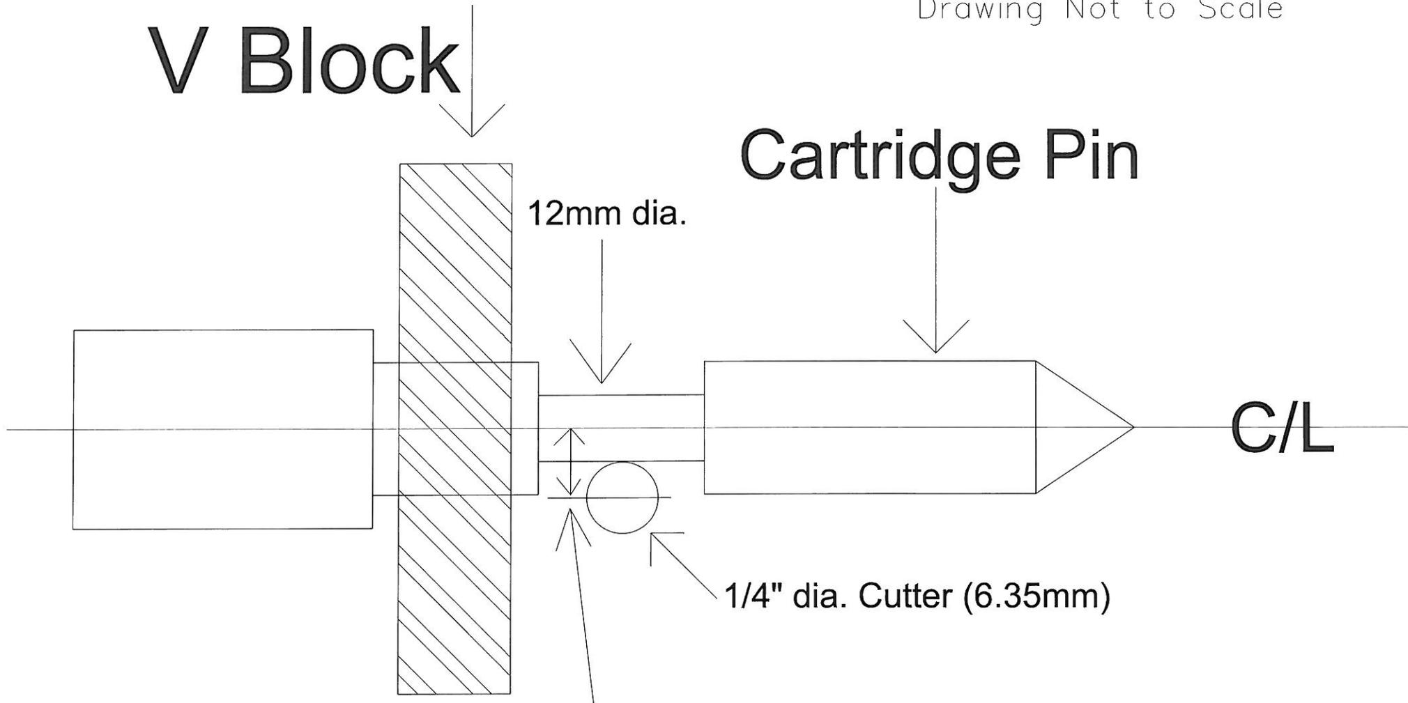
$12\text{mm} + 6.35 = 18.35 / 2 = 9.175$  (radius) Y Offset Tool Compensation
