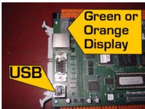
If your machine has been upgraded to USB interface with a new Baldor electronics card (NextMove/NextStep), then the serial plate name may differ to those in the software list.
