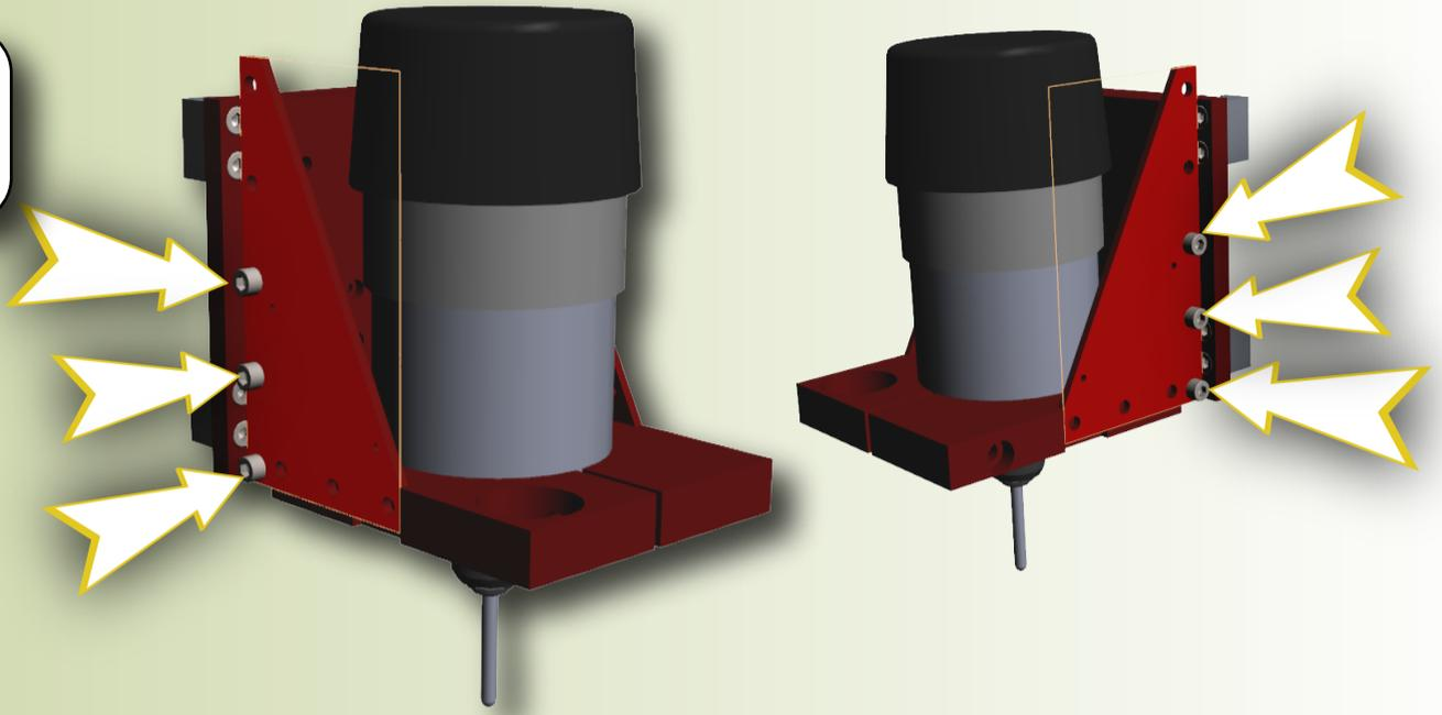
Slide motor and mounting plate up or down until inline with required set of holes (at 35mm increments)
