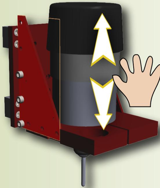
Re-fit and tighten the 6 screws
