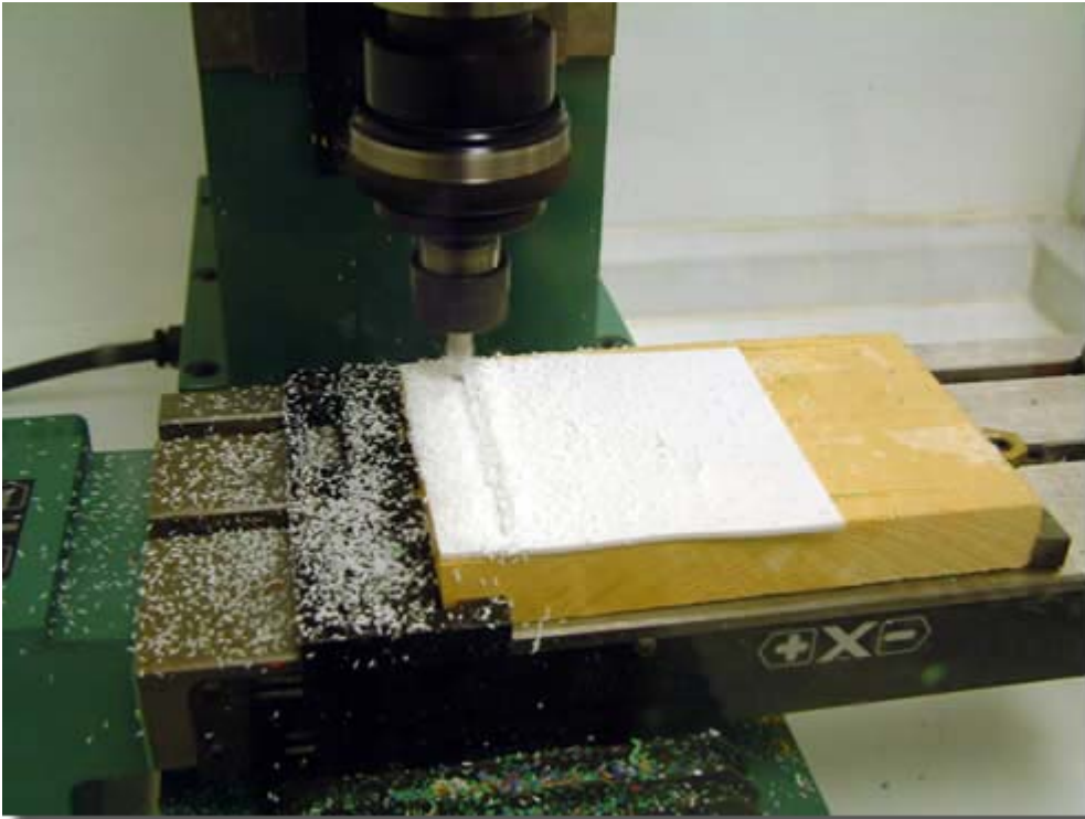
Above: Temporary machine table held using miteebite clamps on a Denford Novamill.
